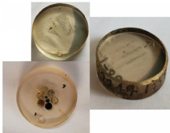
*For LG-SIMS instruments, all grains of interest must be located close to the centre of the mount and to the standard grains to avoid holder edge effects. When analyses are done far away from centre and standards, they can be biased and inaccurate. RM = reference material.*
