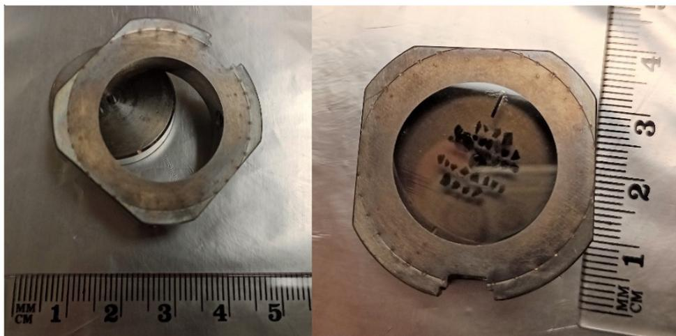
The electrical conductivity on the surface of the sample must be optimised by polishing the sample flat to remove relief (different in height between the resin and the grains of interest). Relief can cause some instability during data acquisition and must be minimised.
