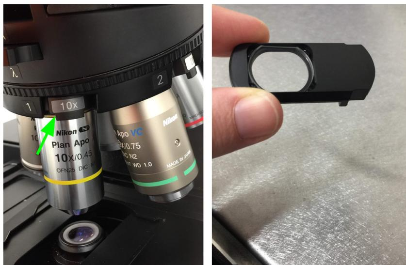
*The DIC Nomarski prism is inserted above the objective to converge the light after it passes through the sample*
