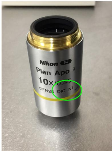
*This objective is capable of DIC imaging, as specified on the objective (green outline).*
